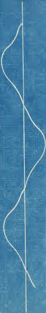
Fig. 27. Wave Form of the Quadrature Component in the Secondary Circuit of Transformer, as Determined by the Ross Wave Tracer. 20 cycles, Fall 1943.
